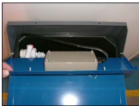
Figure 28 - Removal Of Inclined Panel
