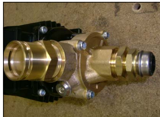
Figure 34 - Non Return Valve Fitting Location On Pump
