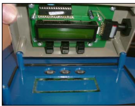
Figure 30 - Assembly Of Display PCB In Enclosure
