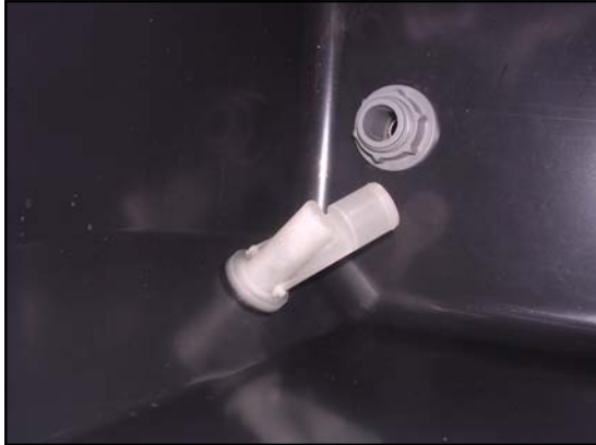
Figure 31 - Level Switch In Tank
